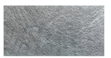
drainage and protection properties. Typar® is a non-woven fabric with remarkable strength and a wide range of application options. It performs well even in very difficult conditions, in road construction, both in dry areas and in degraded areas.
